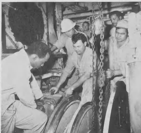
Oil Movements personnel are shown here at work on board the "Esso San Nicolas." At left, the clutch gets new shoes. At right, Henry Orman (c) gets assistance during work on cylindrical clutch drum. Supervising the job (at rear right) is Antero Gil.
